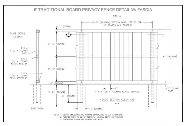
Beveled posts can extend above the top header and trim by up to 2 inches (i.e. Phase 7 standard)
